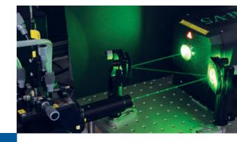
Traceable calibration of counting efficiency according to ISO 21501-4
