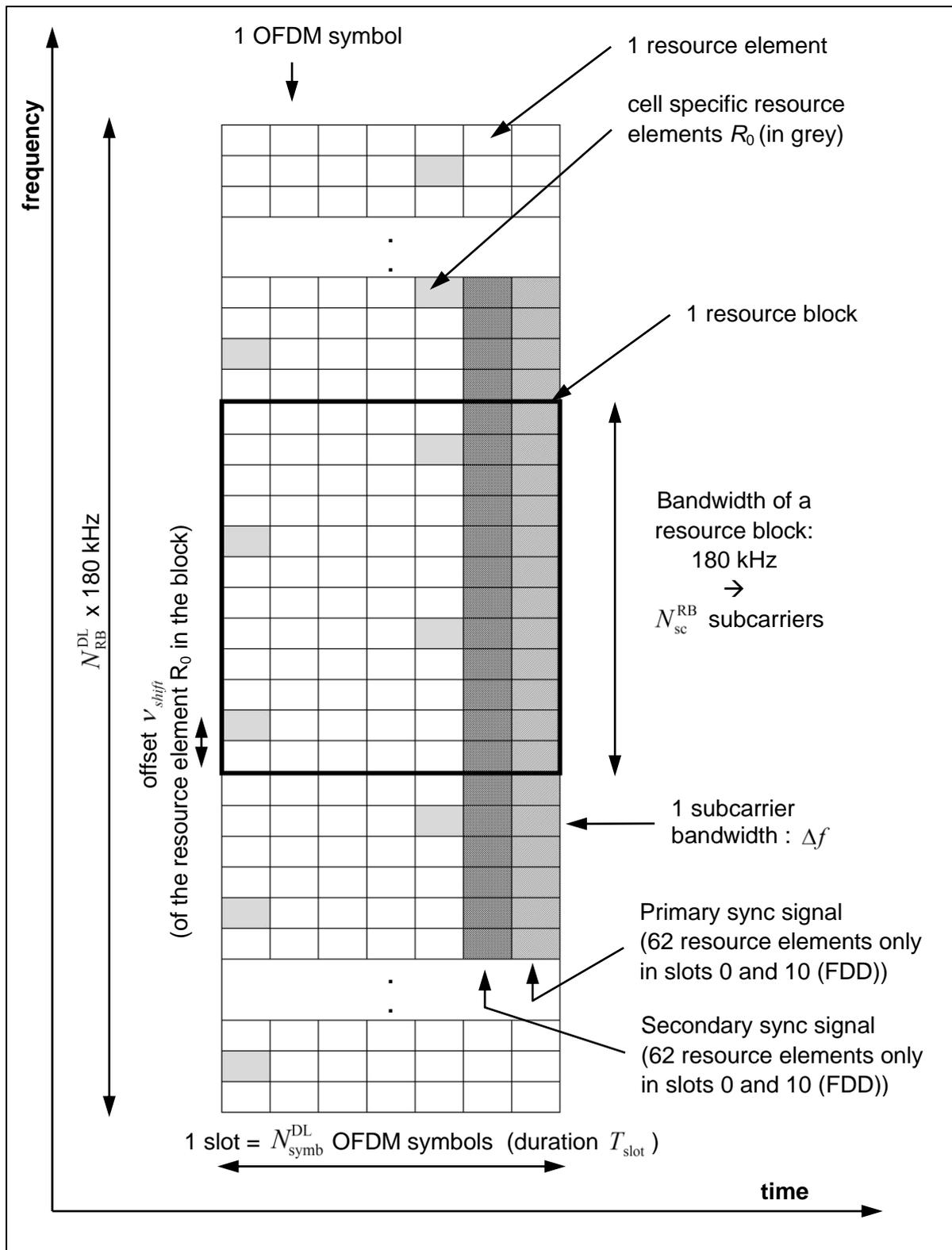
Figure A1: LTE downlink resource grid (reproduced from [6]).
